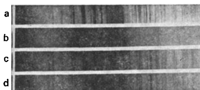
FIG. 1. Guinier X-ray diffraction photographs of crystalline and comminuted digoxin: (a) Swiss Standard digoxin, (b) Swiss Standard ball milled, (c) and (d) Swiss Micronized mortar ground.
